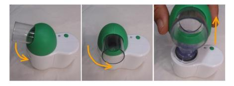
The transducer may now be immersed in warm soapy water for routine cleaning or immersed in Rely+On<sup>TM</sup> Perasafe<sup>TM</sup> solution for a period not exceeding 10 minutes. After cleaning/disinfection, the transducer should be rinsed in distilled water and dried.
